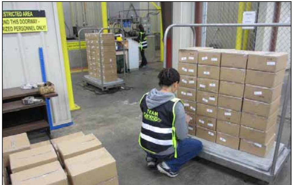
Staff is applying trace-back labels to each produce box before entering the irradiator.
